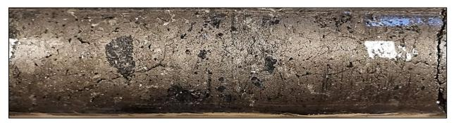
Figure 1: Massive pyrrhotite-pentlandite-chalcopyrite with coarse grained pentlandite and rounded clasts of peridotite, from a 0.3 m sample that returned 2.23% Ni, 0.15% Cu, 0.20% Co, 176.83 m, 23RAN002. NQ diameter drill core.
