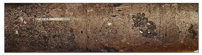
Figure 2: Massive and net-textured pyrrhotite-pentlandite-chalcopyrite with coarse pentlandite loop textures and rounded clasts of peridotite, from a 0.3 m sample that returned 1.71% Ni, 0.26% Cu, 0.15% Co, 176.54 m, 23RAN002. NQ diameter drill core.
