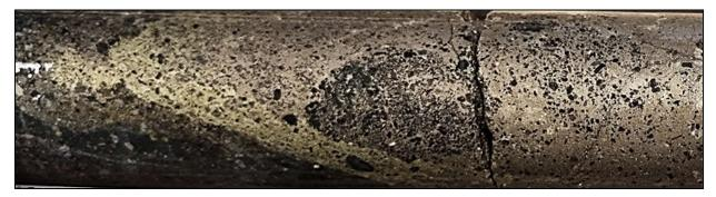
Figure 3: Massive pyrrhotite-pentlandite-chalcopyrite lens with sharp, cross-cutting contact to host peridotite unit. Note the fractionated chalcopyrite rich zone at the contact with host peridotite. From a 0.6 m sample that returned 1.51% Ni, 0.37% Cu, 0.15% Co, 180.0 m, 23RAN002. NQ diameter drill core.
