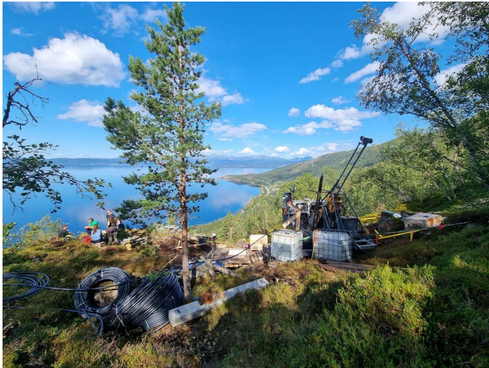
Photo: Drilling contractor Arctic Drilling conducting helicopter supported diamond core drilling at Råna.
