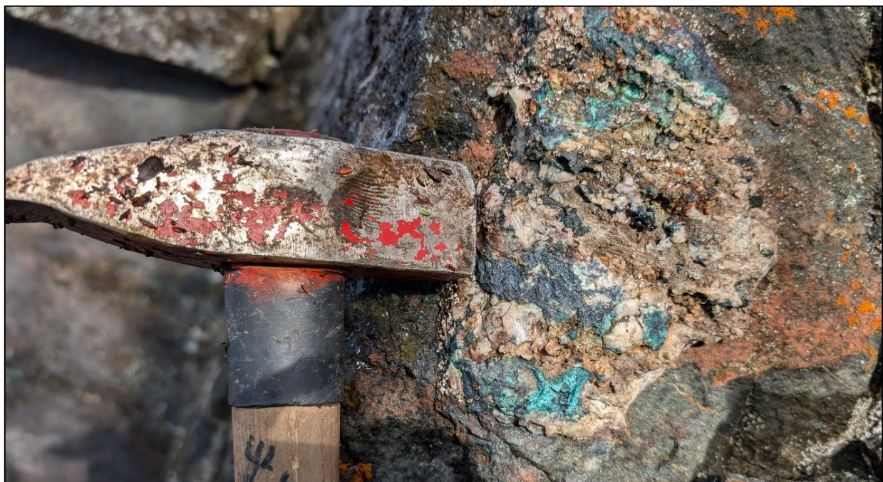
Plate 2: Chalcocite-bornite-quartz vein hosted in amphibolite. 29.7% Cu, 0.01% Ni, 1.1 g/t Au, 53 g/t Ag, 0.54 g/t Pd, 0.02 g/t Pt. Porsanger area, sample 14398.
