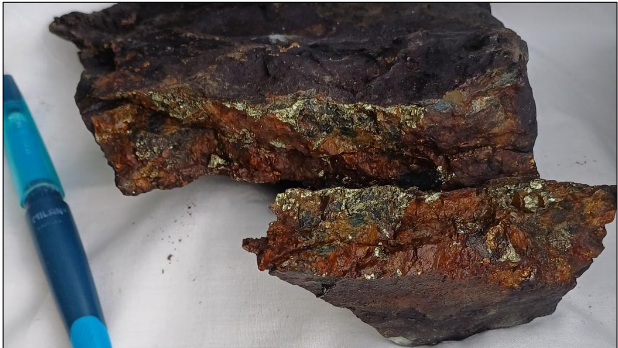
Plate 3: Chalcopyrite-quartz vein hosted in paragneiss. 4.4% Cu, 0.01% Ni, 1.8 g/t Au, 0.50 g/t Pd, 0.06 g/t Pt. Virdnechokka area, sample 14508.
