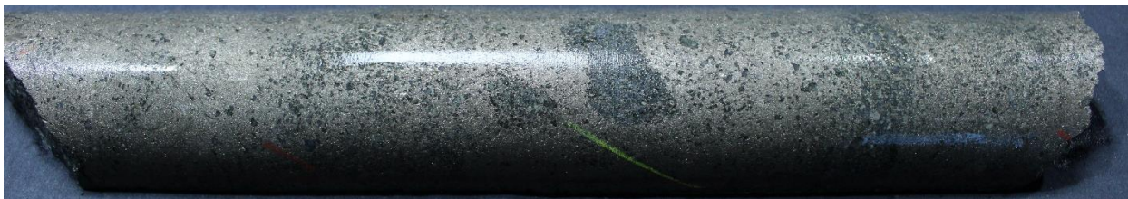
Plate 1: Massive pyrrhotite-pentlandite-chalcopyrite with rounded clasts of entrained norite, from a 0.64 m sample that returned 1.6% Ni, 0.2% Cu, 0.15% Co from 179.50 m, 24RAN010. NQ diameter drill core.
