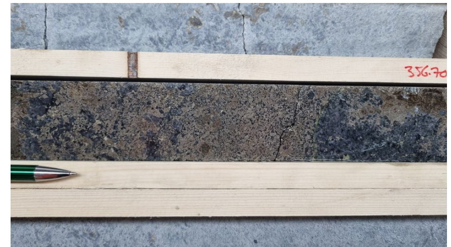
Plate 4: Massive pyrrhotite-pentlandite-chalcopyrite hosted by medium grained pyroxenite from a 0.54 m sample that returned 3.7% Ni, 0.20% Cu, 0.15% Co from 361.0 m, KUSK0015 (RTX drilling).
