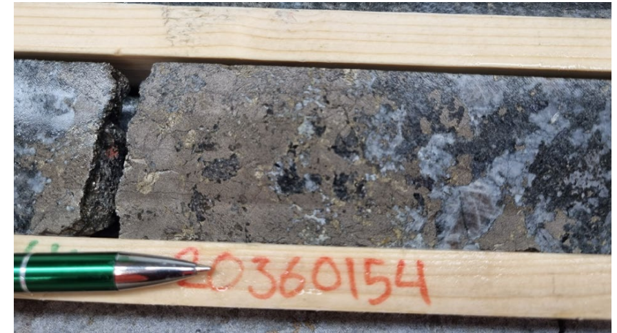
Plate 3: Massive and blebby pyrrhotite-pentlandite-chalcopyrite hosted by coarse grained gabbro from a 1.48 m sample that returned 1.8% Ni, 0.2% Cu, 0.08% Co from 273.22 m, KUSK0015 (RTX drilling).
