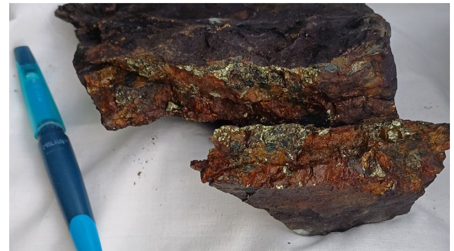
Plate 2: Chalcopyrite-quartz vein hosted in paragneiss. 4.4% Cu, 0.01% Ni, 1.8 g/t Au, 0.50 g/t Pd, 0.06 g/t Pt. Viridnechokka area, sample 14508.
